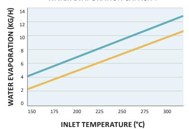
Outlet temperature at 70 °COutlet temperature at 100 °C
