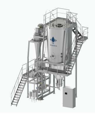
The SD3150 is produced in sanitary design following the GMP guidelines; including state-of-the-art solutions regarding safety and cleaning. The SD3150 is equipped with a sophisticated PLC based control system. All parts in contact with product are stainless steel and all elastomers are food grade approved. Because of the SD3150 size, it is foreseen to be installed in an existing building layout.
