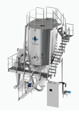
The SD3150 is produced in sanitary design following GMP guidelines and includes state-of-the-art solutions regarding safety, easy cleaning and a sophisticated PLC based control system. All parts in contact with product are made in stainless steel and all elastomers are food grade approved. Due to the size of these spray dryers they are foreseen to be installed in the existing building layout.
