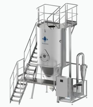
The SD2000 is produced in sanitary design following GMP guidelines and includes state-of-the-art solutions regarding safety, easy cleaning and a sophisticated PLC based control system. All parts in contact with product are made in stainless steel and all elastomers are food grade approved. All plants are skid-mounted, FAT-tested and pre-wired which minimise installation time and costs.
