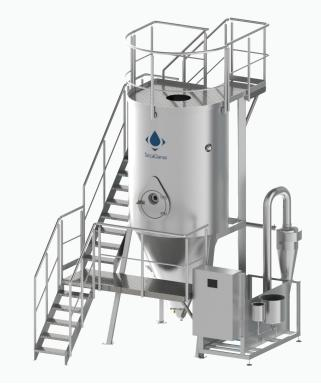
The SD2000 is produced in sanitary design following GMP guidelines and includes state-of-the-art solutions regarding safety, easy cleaning and a sophisticated PLC based control system. All parts in contact with product are made in stainless steel and all elastomers are food grade approved. All plants are skid-mounted, FAT-tested and pre-wired which minimise installation time and costs.
