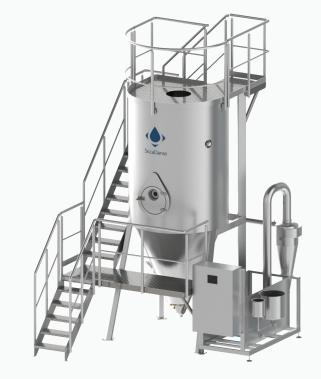
The SD1600 is produced in sanitary design following GMP guidelines and includes state-of-the-art solutions regarding safety, easy cleaning and a sophisticated PLC based control system. All parts in contact with product are made in stainless steel and all elastomers are food grade approved. All plants are skid-mounted, FAT-tested and pre-wired which minimise installation time and costs.
